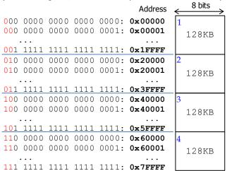
✓ Sketch the circuit that: i) addresses the memory chips, and ii) enables only one memory chip (via CE: chip enable) when the address falls in the corresponding range. Example: if address=0x2FFFF, → only memory chip 2 is enabled (CE=1). If address=0x6ABCO, → only memory chip 4 is enabled.
